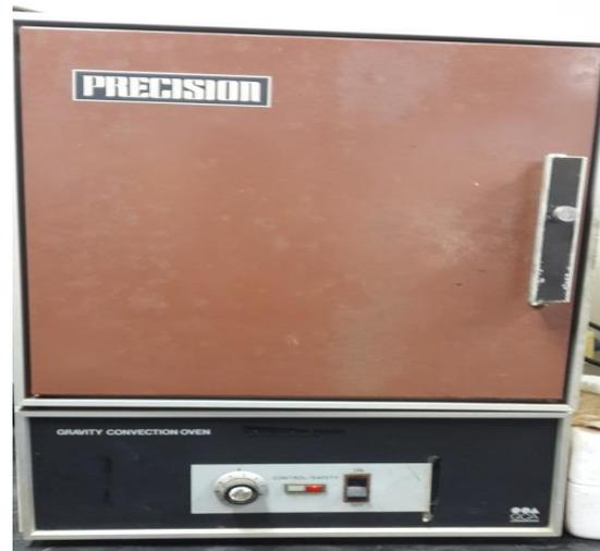
**Figura 3.6** Estufa Gravity Convection Oven, modelo 16, marca Precision.
