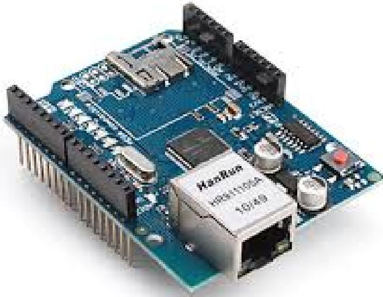
**Figura 3.1:** Placa Arduino Ethernet Shield
