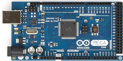
Figura 2.9: Arduino Mega 2560
